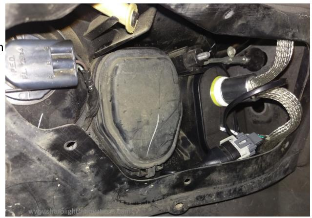
8. Remove the low beam bulb retainer by removing the two T-10 screws. Keep the retainer (it will be re-used).
