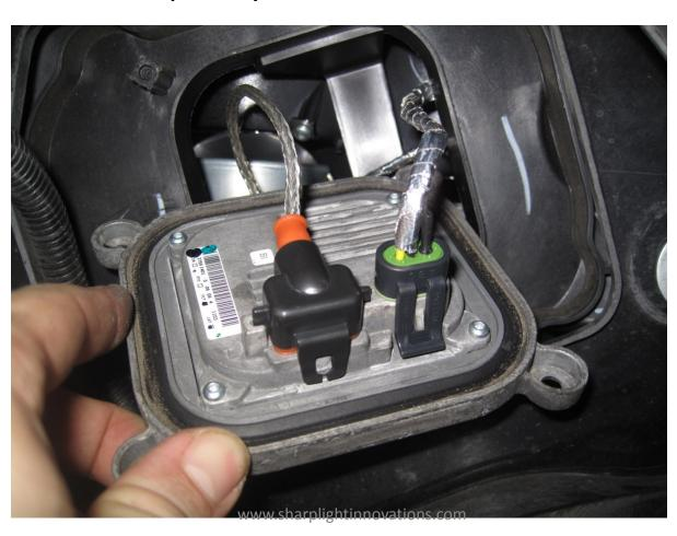
10. Insert the D2S Adapter from the back-side of the headlight as shown. Reach in from the underside to locate the connectors and gently pull them through the opening as shown.
