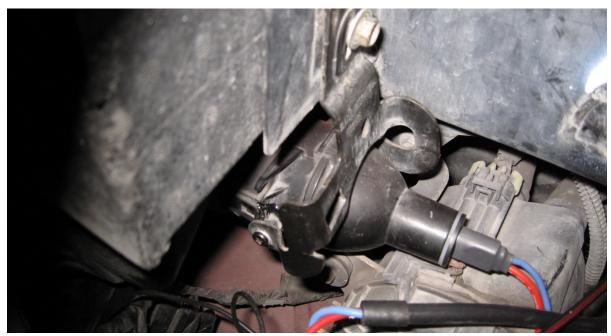
• If you purchased a replacement HID fog light housing (Hella System) to replace your factory fog lights, use a 10mm socket to remove the factory fog light bracket, then a 7mm to remove the factory fog light. Mount the new fog light with the supplied hardware.
