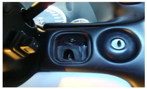
6) Release the locking tabs on the HVAC vent and gently push it backwards. Remove the knee bolster (some wiggling and prying may be required, but don't force it)
