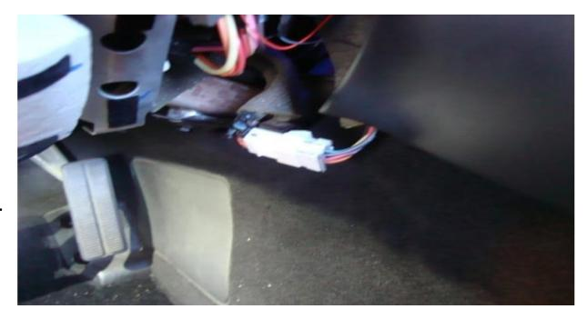
8) Turn the ignition on and check the function of the harness and lights. If everything's good, tuck the harness behind the dash and reverse the dis-assembly process to put everything back together.
