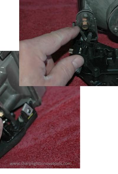
9. Generously lubricate the factory headlight adjustor gearboxes with WD-40, PB blaster or other penetrating lubricant. (failure to do this may result in the brass rod breaking when trying to aim)
