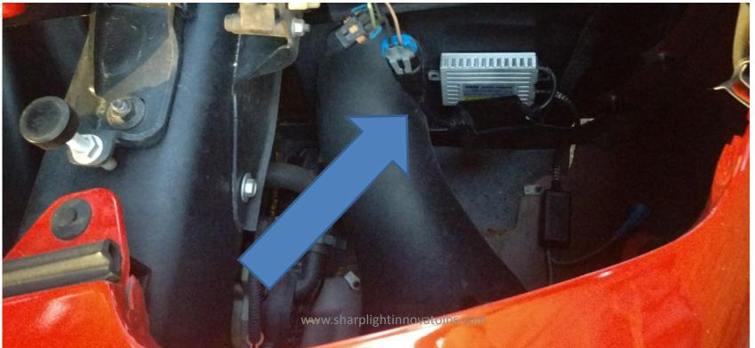
20. The small relay harness with male and female headlight connections installs on the passenger side only between the factory low beam connector and HID ballast as shown. Make sure the polarity is correct on the connections (black wire should line up with the (-) symbol on the ballast connector and the black wire on the factory connector.
