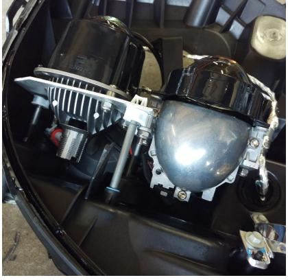
12. Connect the quick connect link between the projectors. Connect the factory H9 connector to the split pigtail to the high beams and projector. (make sure the black wires line up at the connector) Connect the 3-pin factory connector to the wires coming out of the back of the Black LED projector
