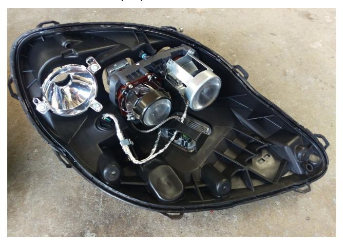
10. Locate the HID ballast on the bottom of the headlight and remove the 4 screws holding it in place. Remove the HID ballast. The 3-pin connector with the green seal will be reused. Remove the output connector. Remount the HID ballast. It serves as a dust seal.
