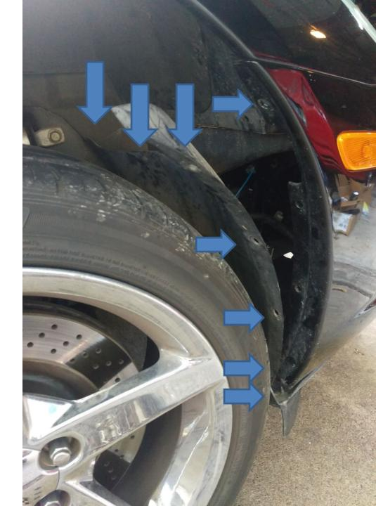
4. Remove the Torx 15 screws along the fender.
