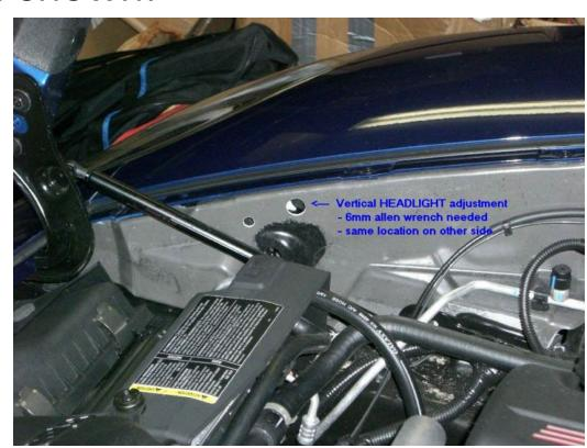
2. At a distance of at least 15 feet (ideally 20+) adjust each headlight until the pattern looks like the pictures. The left side of each beam should be no more than 24" from the ground for cars with factory ride height.
