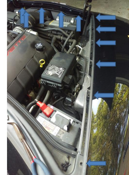
6. Firmly lift the front bumper to reveal an additional Torx 15 screw on the fender. Remove this screw.
