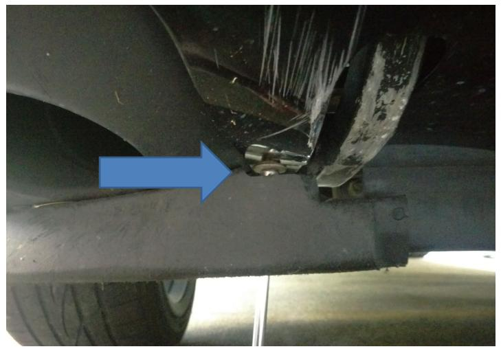
3. Remove the plastic retaining pins shown here. (ZO6 and ZR1 cars also require removal of wheel leading-edge splash guards to access these pins)
