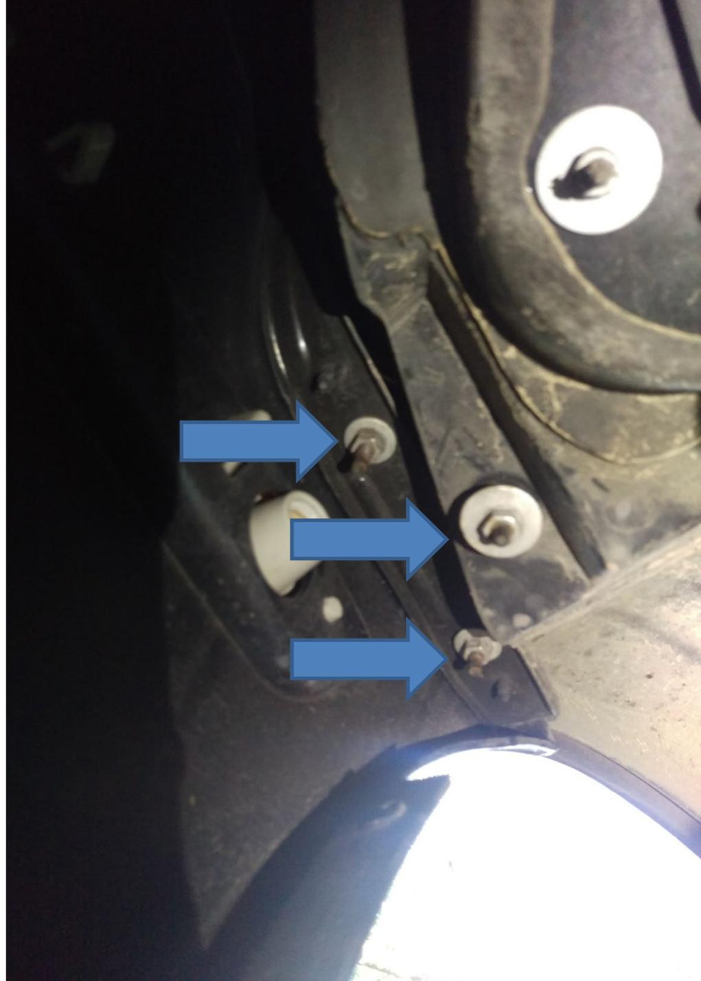
8. Three 10mm nuts with large washers hold the headlight in place. Remove these nuts to release the headlight.
