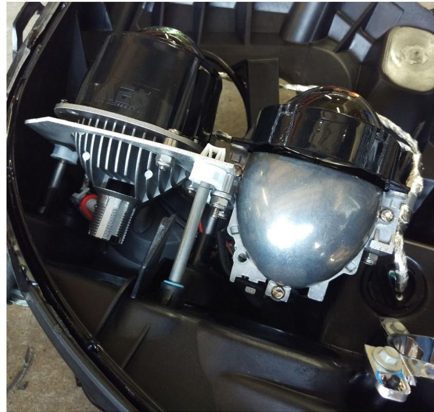
12. Connect the Factory H9 connector to the split pigtail to the high beams and projector. (make sure the black wires line up at the connector) Connect the 3-pin factory connector to the LED driver input. (connector style may vary) Connect the LED driver output to the LED main projector. Tuck away wires.
