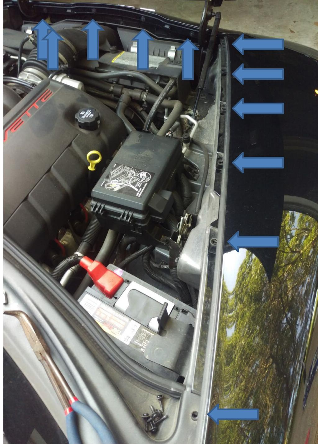
6. Firmly lift the front bumper to reveal an additional Torx 15 screw on the fender. Remove this screw.
