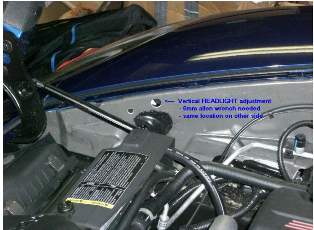
2. At a distance of at least 15 feet (ideally 20+) adjust each headlight until the pattern looks like the pictures. The left side of each beam should be no more than 24" from the ground for cars with factory ride height.
