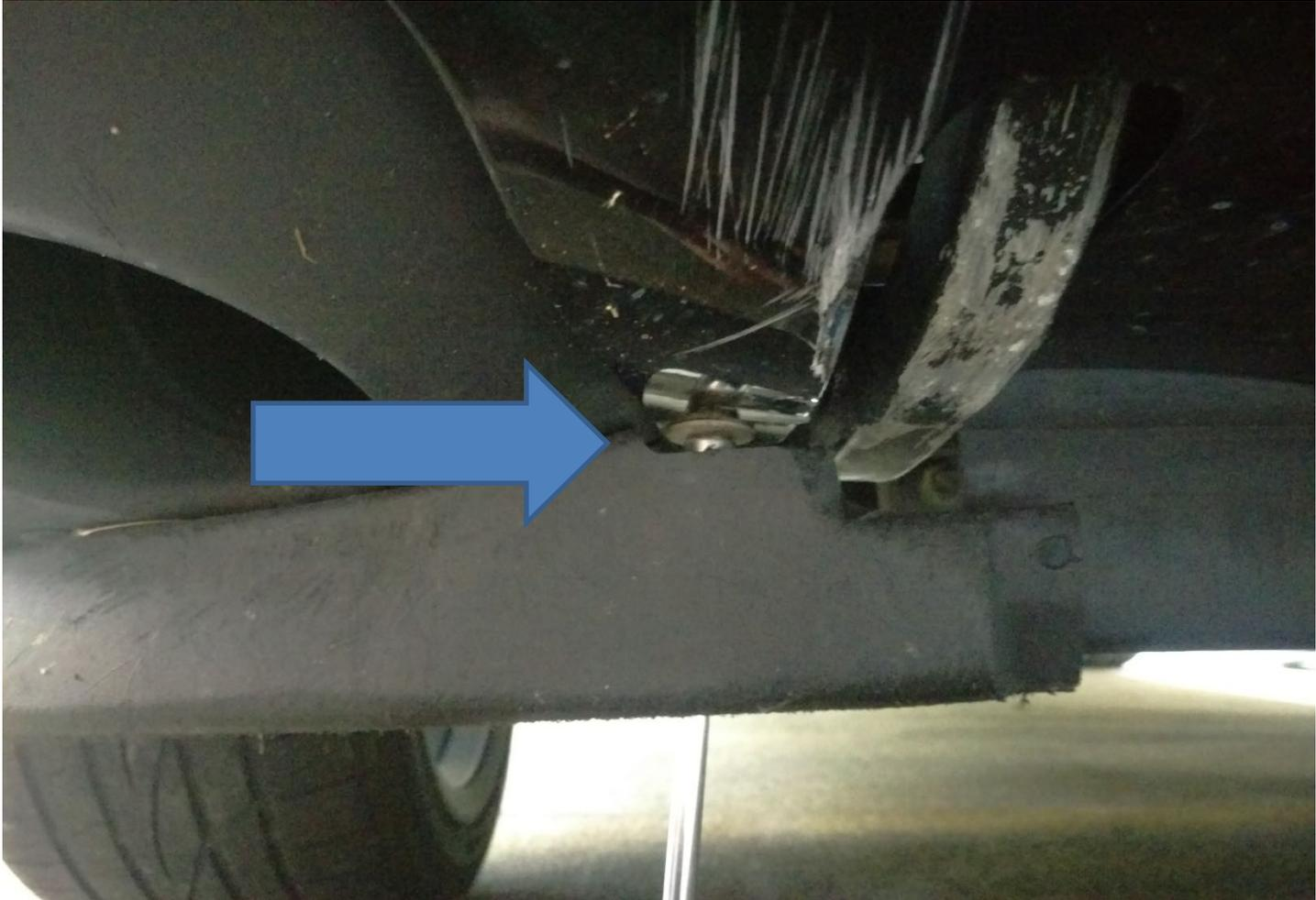
3. Remove the plastic retaining pins shown here. (Z06 and ZR1 cars also require removal of wheel leading-edge splash guards to access these pins)
