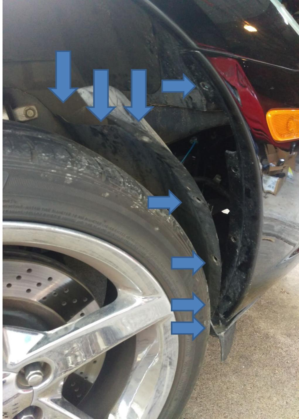
4. Remove the Torx 15 screws along the fender.
