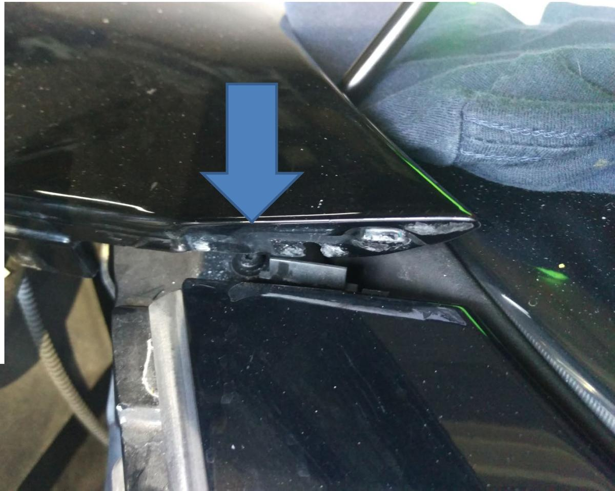
7. From under the car, there are three 10mm nuts that hold the fender to the front bumper. Remove these (A ratchet socket or cordless drill with an extension will help here)
