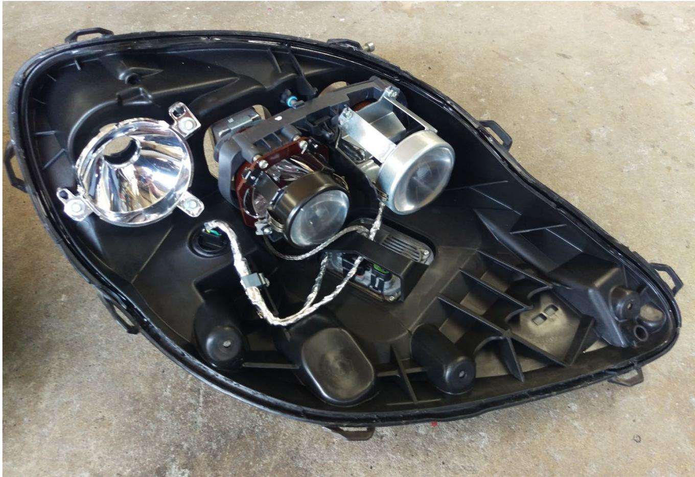
11. Mount the LED driver box to the plastic due plate. (The hardware to mount your box may be different than what is pictured here) Reuse the factory seal as shown and secure the plate with the factory screws
