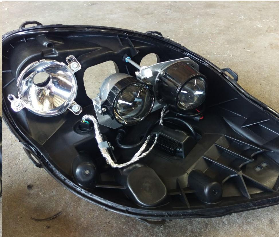
13. If you have the car available, test the light function by plugging into the factory connector. If the test is successful, proceed to installing the new lens (not included) Lens installation best done by a professional or someone with extensive experience.
