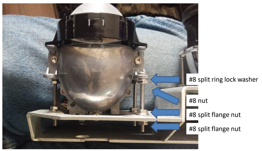
7. Install the High beam projector in the same manner as the Bi-LED projector. The 2.5" screw will be used in the lower mount furthest away from the Bi-LED projector
