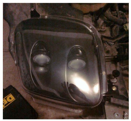
Tighten the nut onto the screw just enough so that the shroud and lens start to press together. Do not tighten any further.
