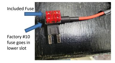
Tap the fuse as shown using the fuse taps supplied with your harness. The leg of the fuse will slide through the tap and back into the fuse socket. The fuse may not seat completely, but as long as you have good contact it will work as intended. Fuse taps install like this:
