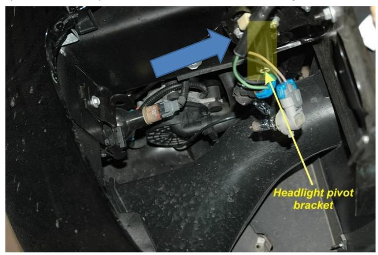
5. There are 5 mounting points that hold the frame in place (shown below) Three 10mm nuts on the wheel well and two 13mm bolts on the frame rail. Make sure to save these as they will be used to mount your new lights. Be Careful not to scratch your paint when removing the frame. (note: the 4"x4" headlight control box shown here bolted to the headlight frame will be removed and the
