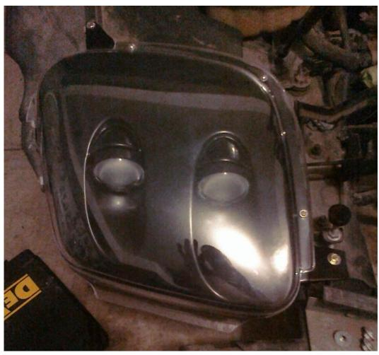
Tighten the nut onto the screw just enough so that the shroud and lens start to press together. Do not tighten any further.
