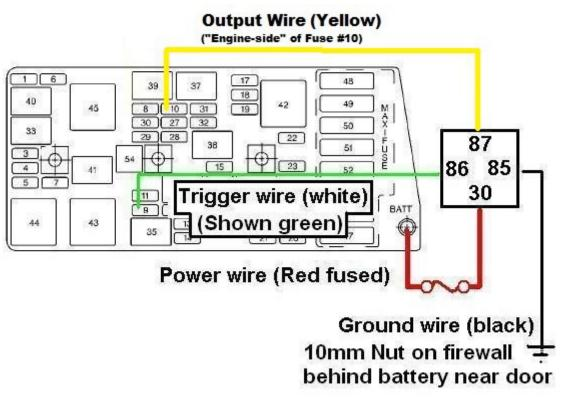
Tap the fuses as shown using the fuse taps supplied with your harness. The leg of the fuse will slide through the tap and back into the fuse socket. The fuse may not seat completely, but as long as you have good contact it will work as intended. Fuse taps install like this:
