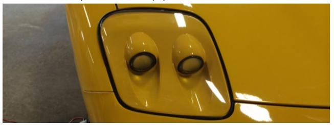
Lens painting - When painting the lens, note how much area you'll need to get an effective beam pattern from the high and low beams. I suggest using painters tape on the lens to mark this area. After painting, remove the painter's tape and shoot the entire lens (including the unpainted section) with clear-coat to minimize the possibility of flaking.
