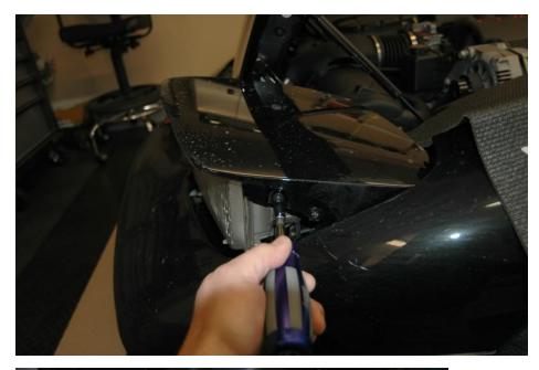
3. Remove the 2 Torx 20 bolts/8mm nuts that are the headlight hinge joint. (It may be beneficial to spray these with WD-40 or similar as they are installed with Blue Lock tight from the factory)
