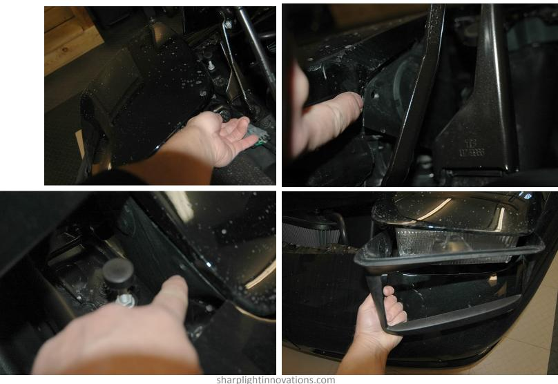
2. Remove the 4 torx 15 screws that hold the headlight cover in place. 2 are on the back and there's one on each side. Remove these and the headlight cover. Be sure not to lose the plastic or metal sleeve for the bolts.
