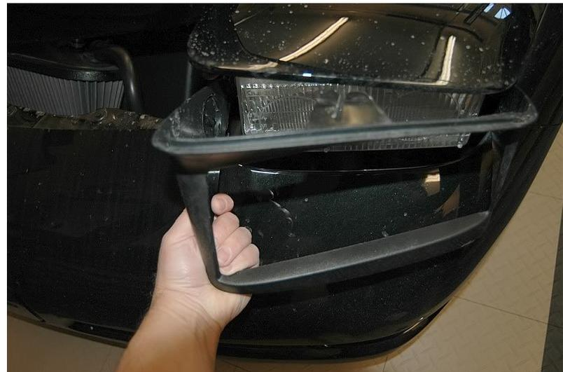
2. Remove the 4 torx 15 screws that hold the headlight cover in place. 2 are on the back and there's one on each side. Remove these and the headlight cover. Be sure not to lose the plastic or metal sleeve for the bolts.
