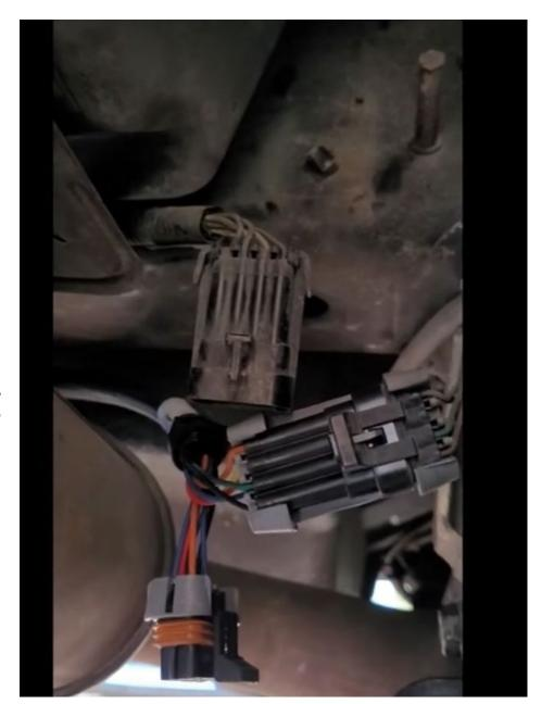
5. Run the other end of the harness up through the same gap the factory harness uses. (between the outer storage bin and frame rail)
