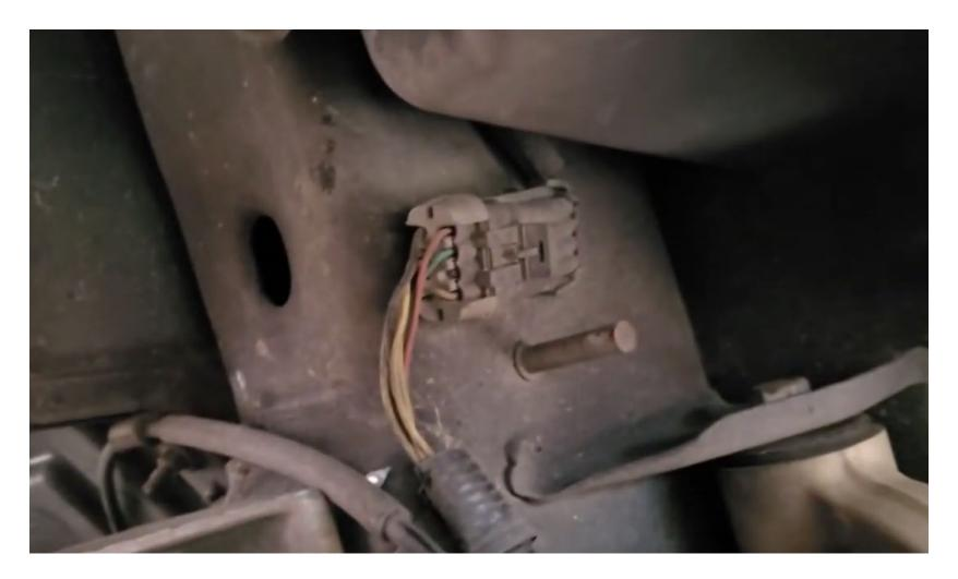
4. Insert the matching male/female ends of your new harness between the factory harness connectors.
