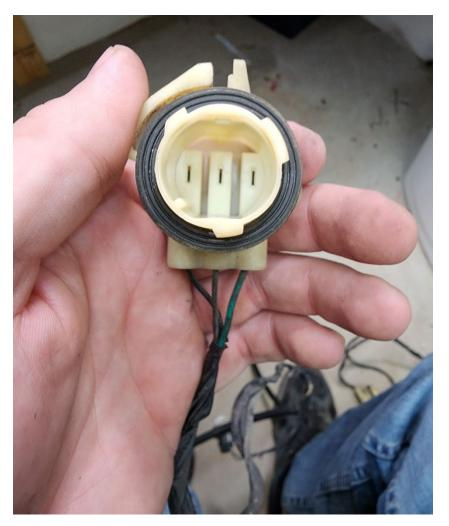
7. Remove the green wire in the "A" position and contact from both sockets. Cut the green wire at the shown location and strip about  $\frac{1}{4}$ " to  $\frac{3}{8}$ " of insulation from the harness side of the green wire. (Discard the ends with the contacts)
