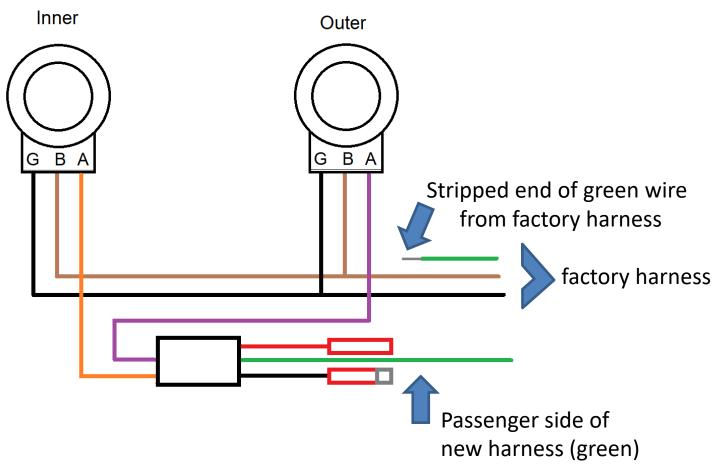
9. Use the posi-tap to tap the black ground wire from the new harness to the black ground wire on one of the sockets. Use the posi-lock to connect the red wire from the new harness to the green wire you previously stripped. Repeat steps 6-9 on the other side tail light
