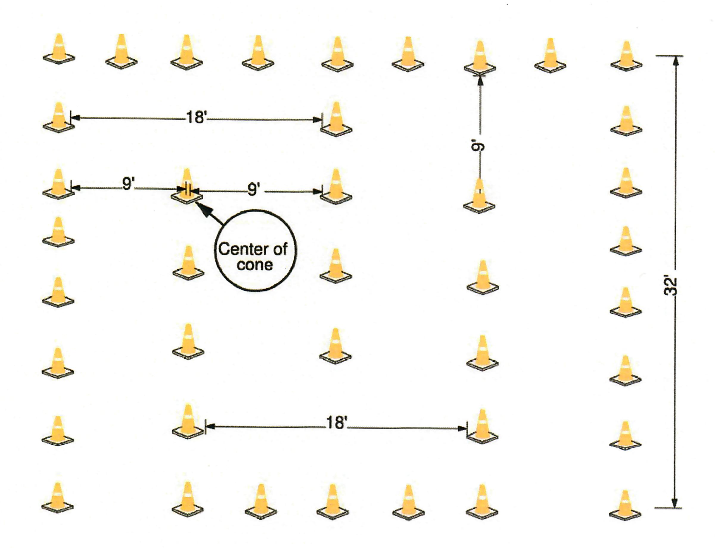
All measurements are from inside of cone to inside of cone except where indicated.
