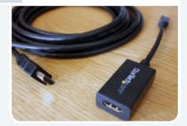
Connect the HDMI cable to the mini display to HDMI adapter
