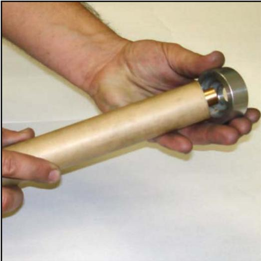
The FireSmith Spindle Removal Tool is designed to both enhance the safety of rocket construction and reduce the effort required to remove a rocket motor from its spindle. The potential hazards and motor damage associated with using clamps, pliers or wrenches to twist a completed motor from a spindle are greatly reduced as well. This tool is quite easy to use by simply following these instructions:
