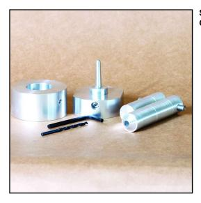
Step 1 Gather the stinger spindle, rammers, drill jig, Allen key and drill bit.
