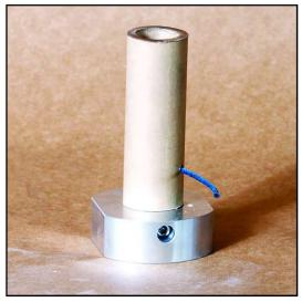
Step 9 Insert the 3" length of Visco fuse into the vent hole.
