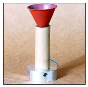
Step 10 Using a small funnel, load one increment of BP fuel into the motor tube.
