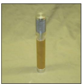
Step 4 Insert the rammer with a twisting motion to help capture the fuse in the rammer bore. Use a dead blow mallet to pack the clay into a solid plug. Typically 4-5 good hits is sufficient. The plug should be approximately 1" in thickness. The correct thickness is attained when the groove machined into the rammer is visible at the top of the tube after ramming.
