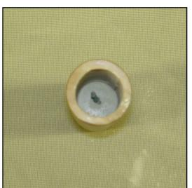
Step 5 Remove the rammer and the base. The black match should be sticking up through each end of the clay plug.
