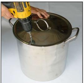
Using the 1/4" bit, drill 4 vent holes in the lid of the stainless pot. Space these vent holes evenly around the lid.
