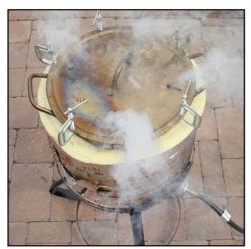
After another 10-15 minutes the volume of smoke being emitted from the vent holes will increase dramatically. This smoke consists of water, saps and various hydrocarbons contained within the wood.
