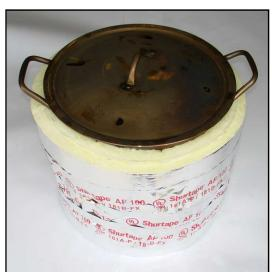
Step 3 Wrap the pot with 2 layers of fiberglass insulation, securing it with aluminum tape. Though this insulation is not absolutely necessary, it
