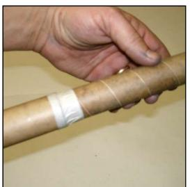
Step 3 Apply a couple wraps of kraft tape around the joint of the motor and heading tube.
