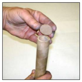
Step 6 Glue a paper or chipboard disc over the end of the heading tube.
