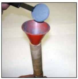
Step 5 Dump 1 tablespoon of dark aluminum into the heading tube.
