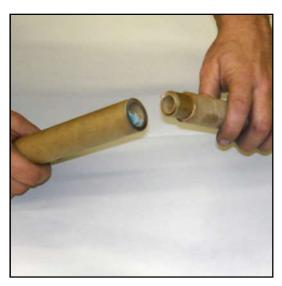
Step 1b With larger motors it may be difficult to locate paper tubes that fit the OD of the motor. In this situation, a section of paper tube with the same ID as the motor may be used. Simply cut a 1" length of tube that fits the ID of both the motor and the heading tube. Glue this tube 1/2" deep into the heading tube.
