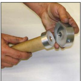
Set the base on the spindle/pressed motor and insert the 1" long cap screw through the base and into the bottom of the spindle.
