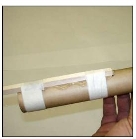
Step 4 Further secure the stick to the motor with a couple wraps of masking or strapping tape.
