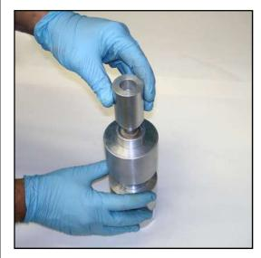
Step 32 Slide the tube extender over the rammer and set aside.
