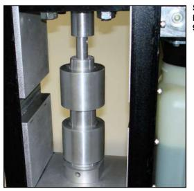
Step 21 Insert the entire assembly into the press and compact the fuel to 8,000-9,000psi.
