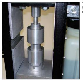
Insert the entire assembly into the press and compact the fuel to 8,000-9,000psi.
