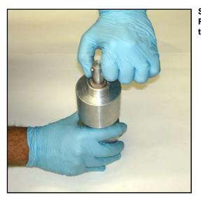
Remove the assembly from the press, insert the "T-puller" and with a light twisting motion, remove the rammer from the motor.
