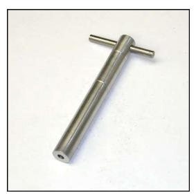
Step 11 Switch to the #2 rammer (the second longest with a flush tip).
