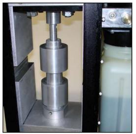
Step 33 Insert the entire assembly into the press and compact the fuel to 8,000-9,000psi. Remove the rammer and repeat steps 30-33 until the motor is filled to within 1/2"-1" from the top of the tube.
