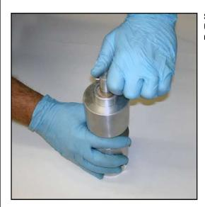
Use the puller and a slight twisting motion to remove the rammer from the motor tube.
