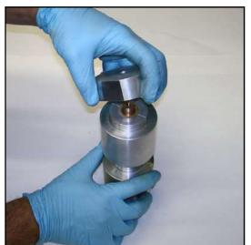
Step 34 Remove the entire assembly from the press. Using a 3/16" hex key, remove the base from the spindle.
