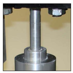
Step 17 Repeat steps 12-16 until the swap-out line is visible above the top of the motor tube after pressing an increment of fuel.
