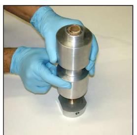
Step 3 Slide the tube & tube support assembly onto the motor spindle.
