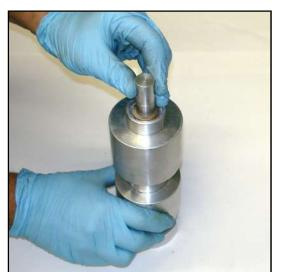
Insert the #4 rammer and seat the fuel with light hand pressure.
