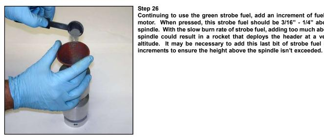
Step 26 Continuing to use the green strobe fuel, add an increment of fuel to the motor. When pressed, this strobe fuel should be 3/16" - 1/4" above the spindle. With the slow burn rate of strobe fuel, adding too much above the spindle could result in a rocket that deploys the header at a very low altitude. It may be necessary to add this last bit of strobe fuel in half-
