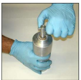
Step 22 Using the puller, apply a slight twisting motion and remove the rammer from the motor tube.
