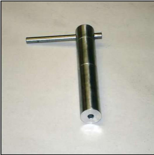
Step 18 Switch to the #3 rammer (the third longest with a flush tip)
