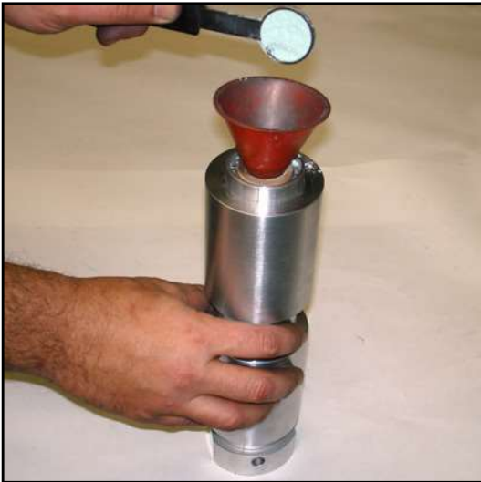
Step 19 Add another increment of non-titanium bearing fuel.
