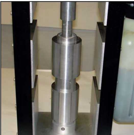
Step 14 Insert the assembly into the press and compact the fuel to 8,000-9,000psi.
