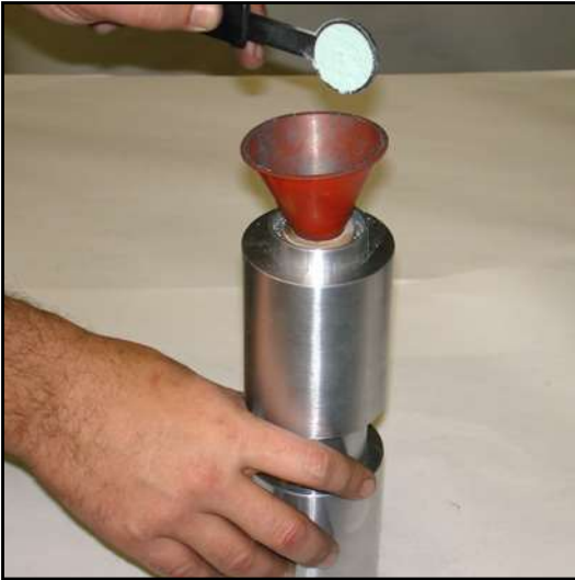
Step 12 Add another increment of non-titanium bearing fuel
