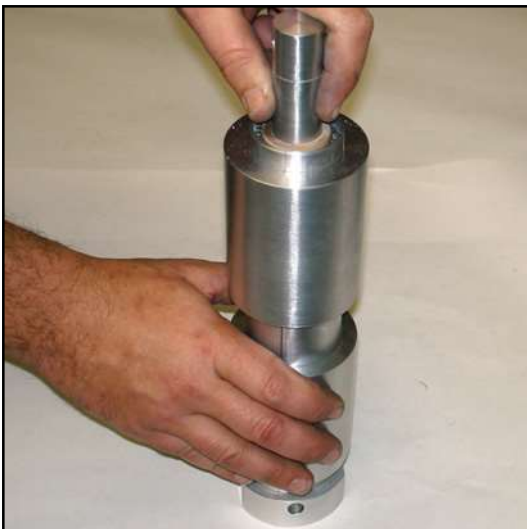
Step 20 Insert the #3 rammer into the motor tube and seat the fuel with light hand pressure.
