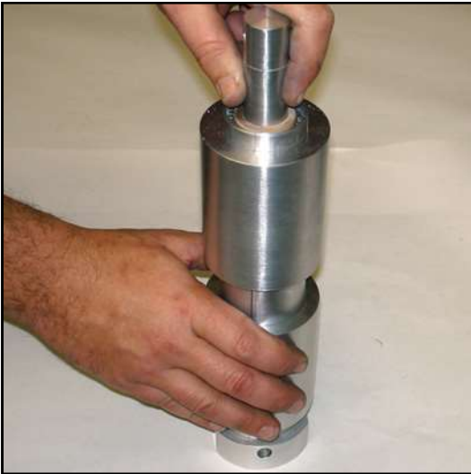
Step 13 Lightly seat the rammer with hand pressure
