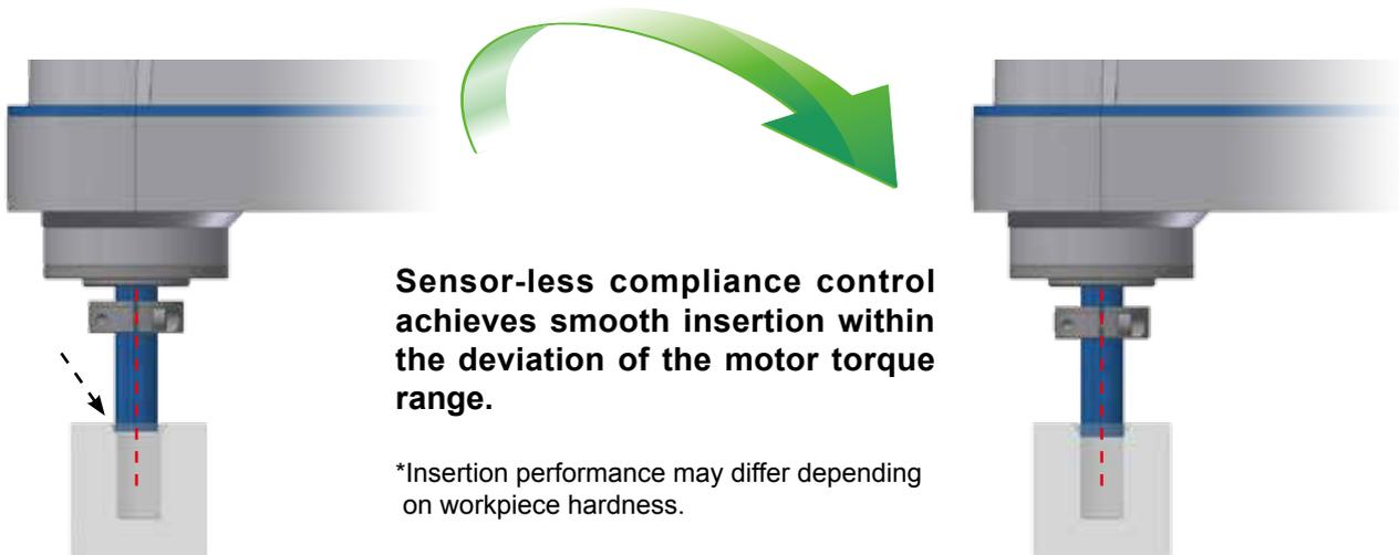
**Sensor-less compliance control achieves smooth insertion within the deviation of the motor torque range.**
