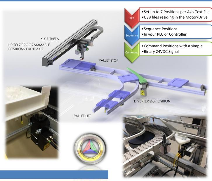
Pallet stops are pre-programmed for 12mm travel. Up Position time is 350ms Down Position time is 750ms
