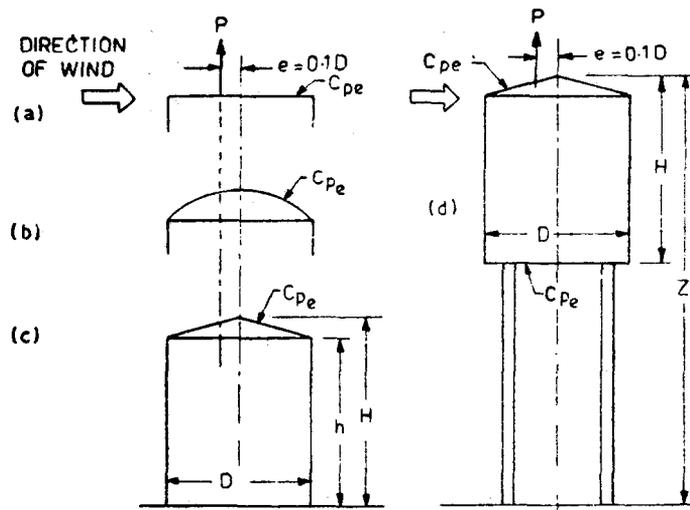
**COEFFICIENT OF EXTERNAL PRESSURE,  $C_{pe}$**
