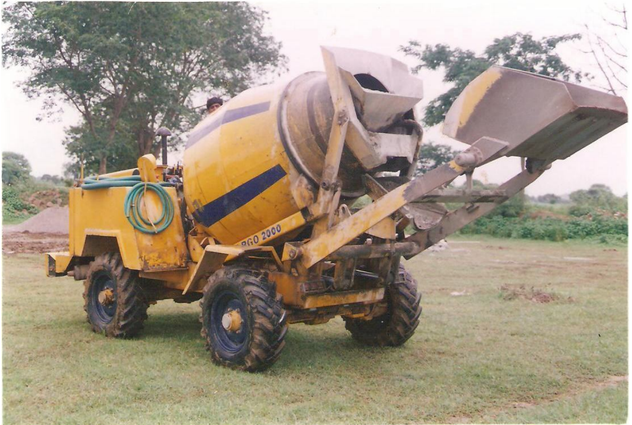
Mobile " Self-Loading, Weigh batching, and Mixing as well as transporting concrete mixer " ( viz mobile B & M Plant )
