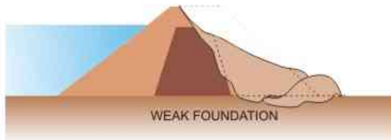
FAILURE OF UPSTREAM SLOPE
