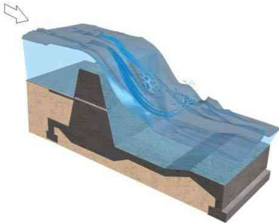
FIGURE 6 . Vertical drop fall
