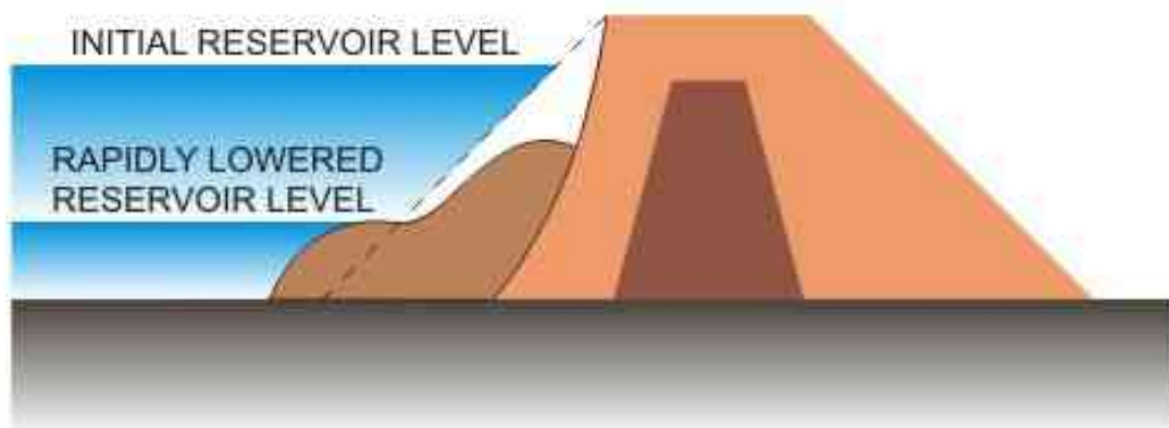
FIGURE 30. Upstream slope failure due to rapid drawdown
