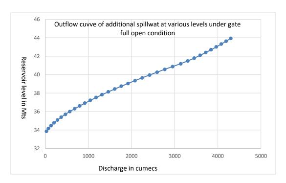
Spillway discharge (free flow) for Rallapadu dam through its 10 Nos old spillway gates for different reservoir levels under full gate open condition has given in tabular and graphical format below.
