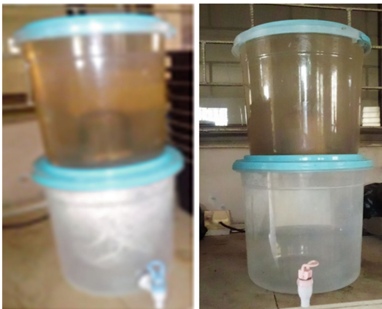
Fig. 12.9 Setup to determine the clogging effect using a filter with a 50 mL/h flow rate. Source Authors
