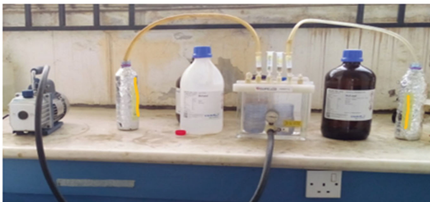
Fig. 12.8 Samples extraction using the solid phase extraction method. Source Authors
