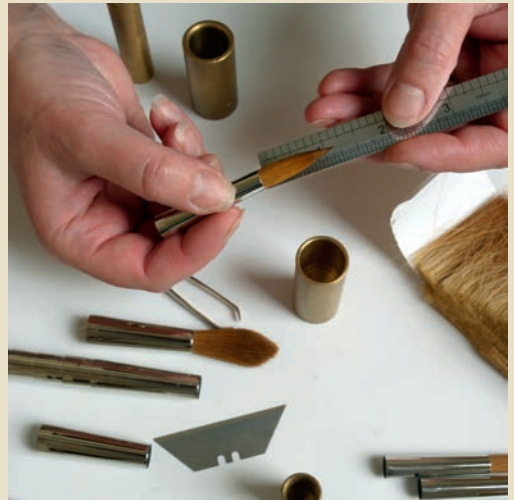
4. Final inspection and measure to check correct 'length out'.
