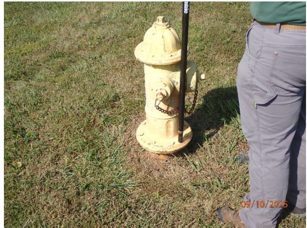
TBM on fire hydrant
