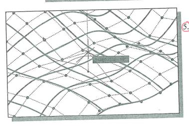
The NURBS surface can now be adjusted by dragging & dropping the available control vertices.
