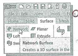
In the *Create* toolbar, activate the **Network Surface** command as shown.
