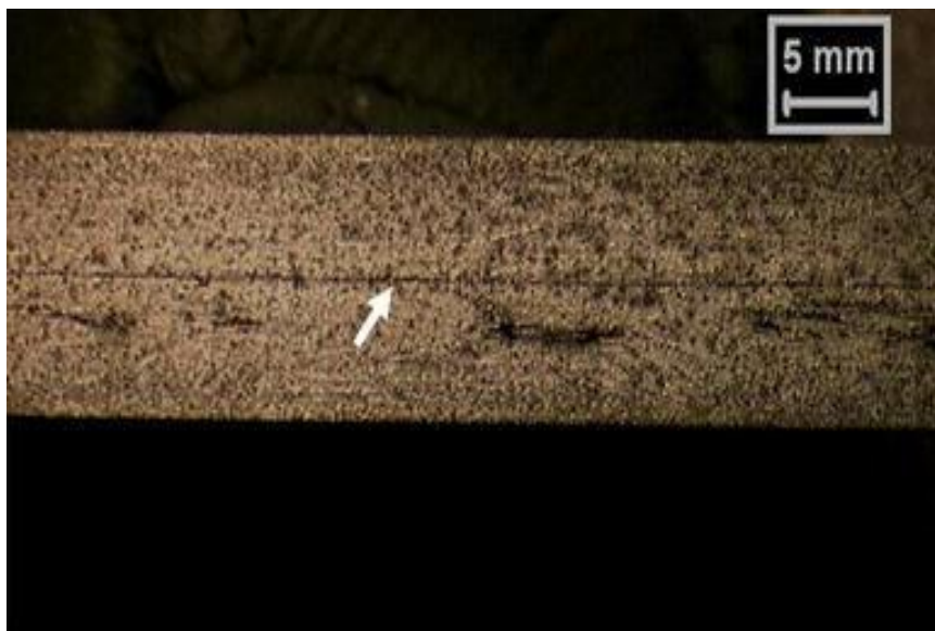
Figure 1. Crack-like defect at slab or billet centerline [2]
