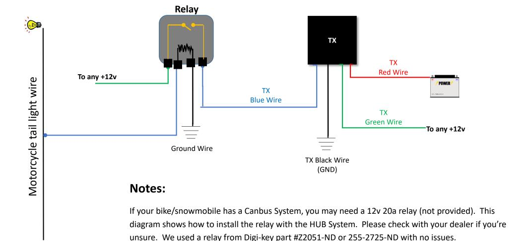
Brake light wire on F800GS and F700 voltage is around 2 volts for tail light. When the brake is applied, this wire gets 12 volts.
