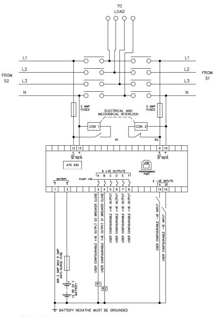
TERMINALS SUITABLE FOR 22-16 AWG (0.6mm - 1.3mm ) FIELD WIRING TIGHTENING TORQUE = 0.8Nm (7lb-in)
