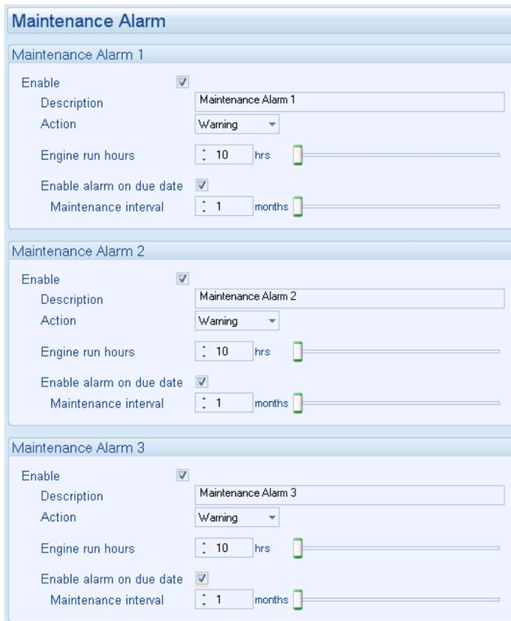
The screenshot displays three configuration panels for Maintenance Alarms 1, 2, and 3. Each panel has the following settings:
