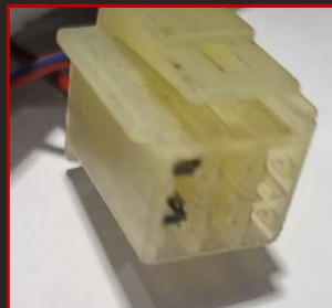
Ecu software flash plug. Don't worry you probably never need to do a software update but its there if you do.
