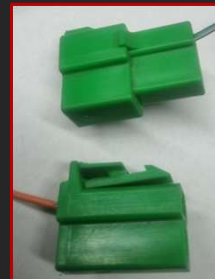
Diagnostic test mode plugs. When connected puts the ECU in test mode and runs sensor, fans, fuel pump, etc. Leave unplugged
