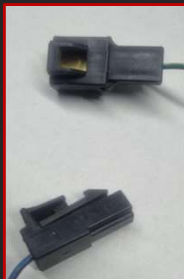
Diagnostic flash code plugs. Google Subaru flash codes which explains. Leave unplugged
