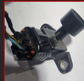
Barometric pressure sensor mount in engine bay
