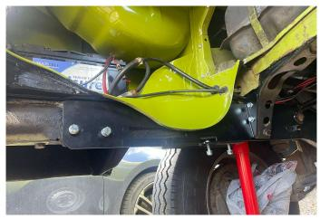
Bolt in both side plates leaving all bolts loose until the engine is fitted then tighten up
