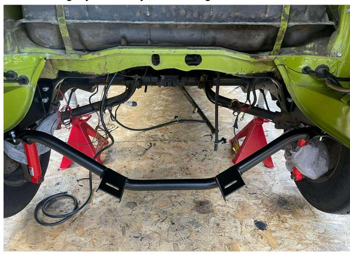
Engine mounting bar shown in its final position, however it should be fitted to your engine before fitting don't try and fit the engine around this
