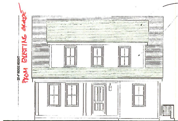
(1) TYPE B-4 & B-5 FRONT ELEVATION Scale: 1/4" = 1'-0"
