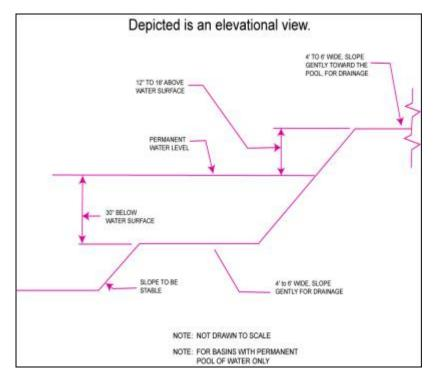
e. Illustration of Safety Ledges in a New Stormwater Management Basin.
