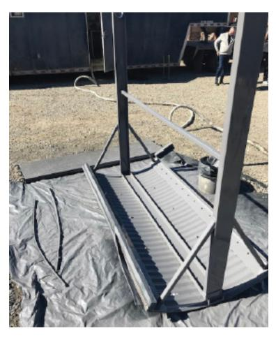
The coating is produced from castor oil and gypsum, and thousands of tanks, steel, and concrete structures have been coated with it, including ship decks. Its high resistance to corrosion has been well demonstrated in frac production water and oil tanks which are often contaminated with the cocktail of chemicals, many of which are corrosive, that are used in that oil extraction process.
