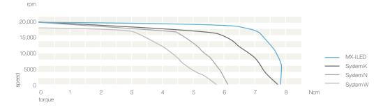
The MX-i LED micromotor is first and foremost a model of stability. It offers great working comfort at both high and low speeds. The high torque of the MX-i LED makes it one of the most powerful micromotors on the market. Depending on the torque needed, the power is regulated and stabilised by the electronic system. This allows the speed to be maintained with great precision throughout the operation.
