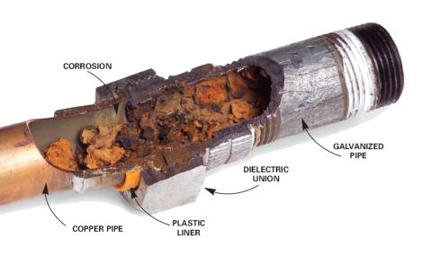
Electrons are lost by the iron, and the iron undergoes rapid corrosion
