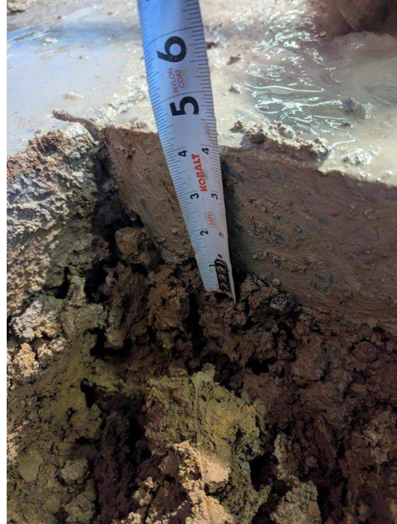
Photo 6: Interior Test Pit TP-2A; view of floor slab thickness
