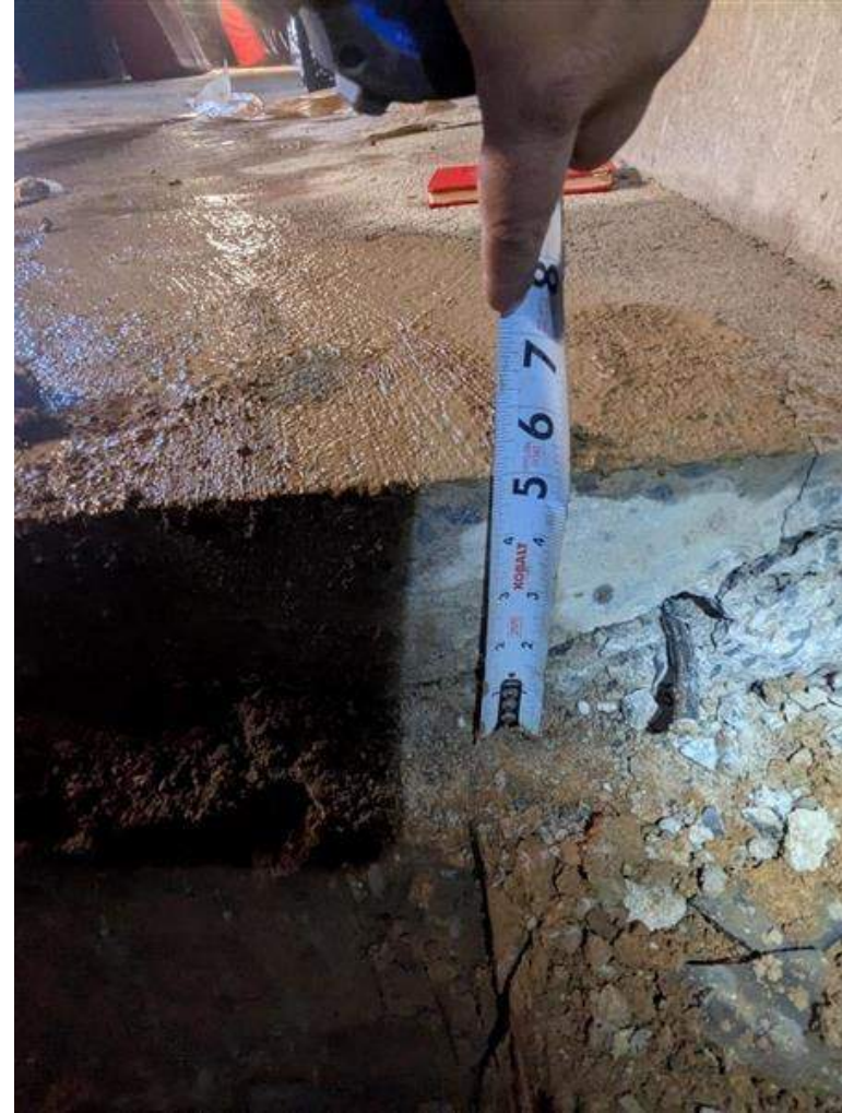
Photo 2: Interior Test Pit TP-1A; view of floor slab thickness
