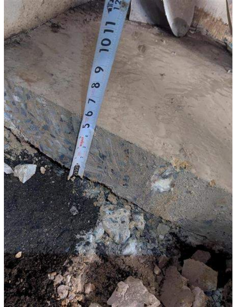
Photo 10: Interior Test Pit TP-3A; view of floor slab thick-
