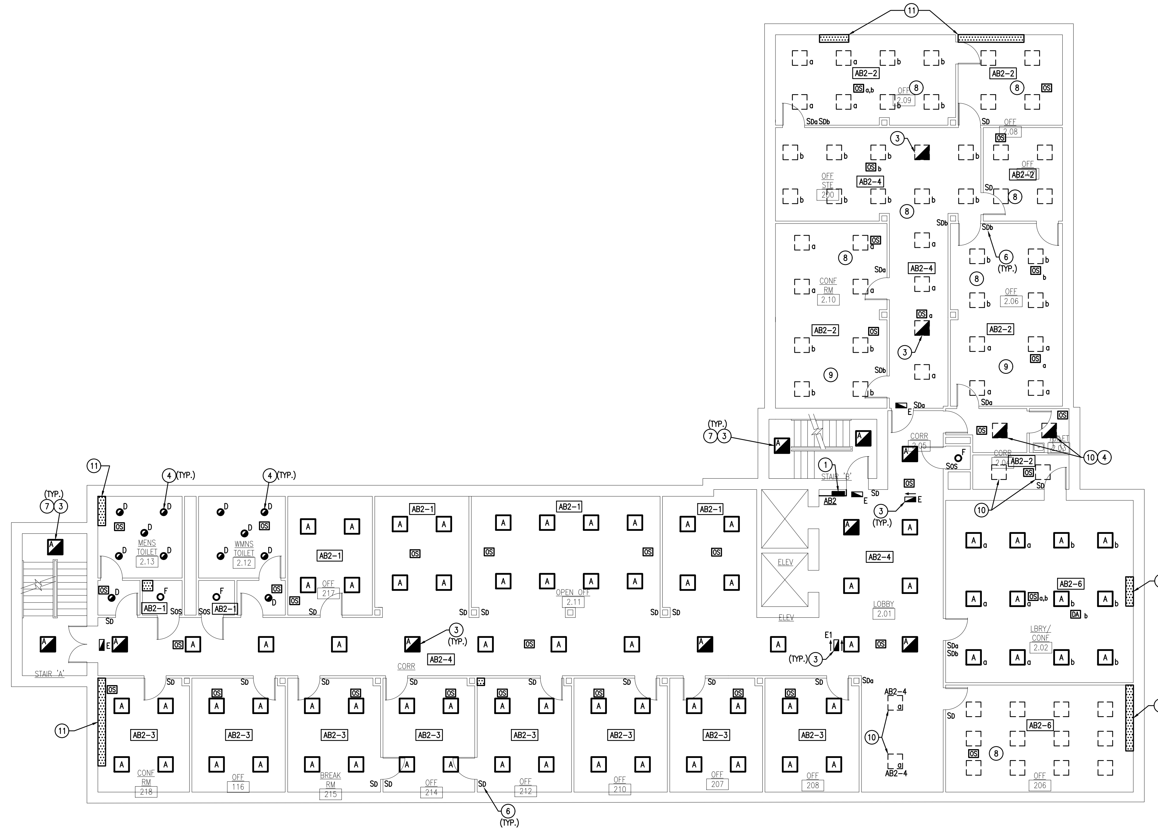
SECOND FLOOR PLAN - LIGHTING SCALE: 1/8" = 1'-0" (2/8)
