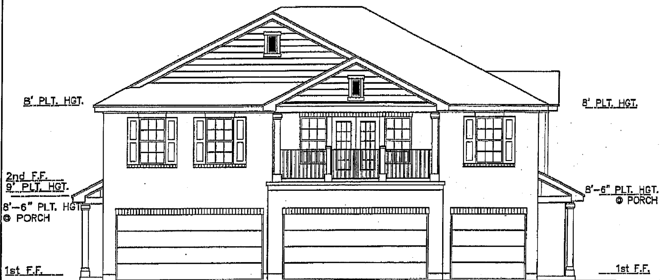
FRONT ELEVATION BUILDING TYPE 4096 RIGHT CONFIGURATION
