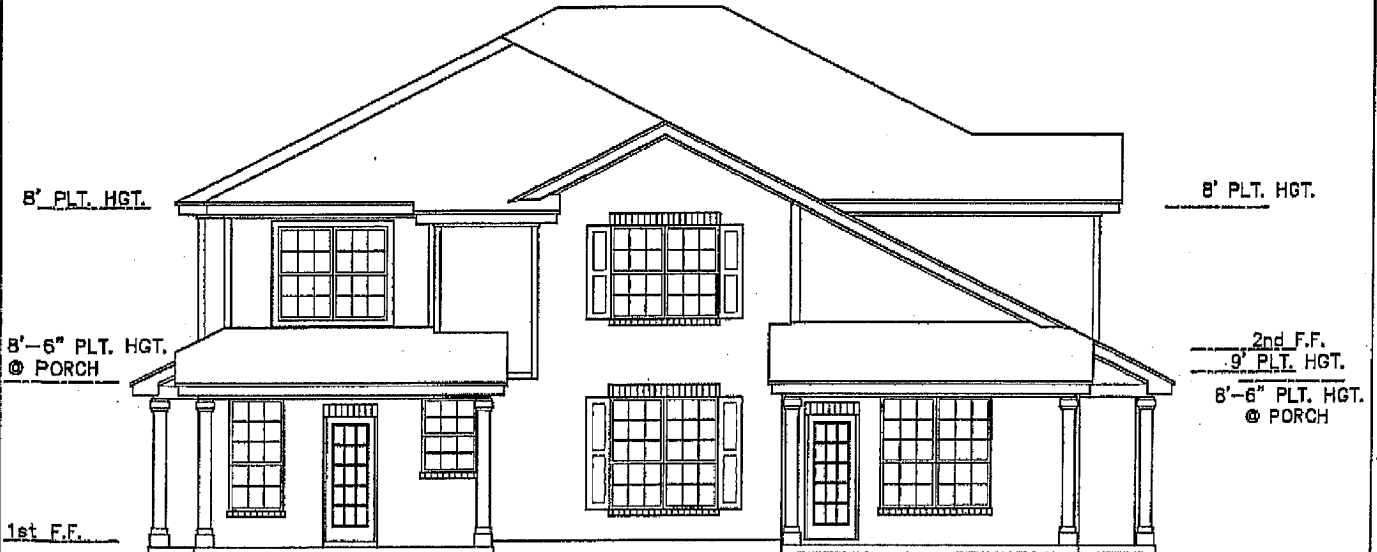
REAR ELEVATION BUILDING TYPE 4096 LEFT CONFIGURATION
