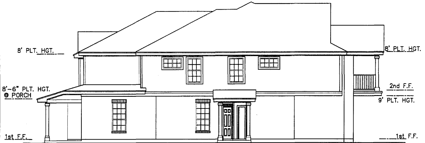
LEFT ELEVATION BUILDING TYPE 4096 RIGHT CONFIGURATION
