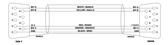
Note: with this cable, in the case of the Expert amplifier off, the Matrix automatically activates the ANT1 in accordance with the Expert manual.
