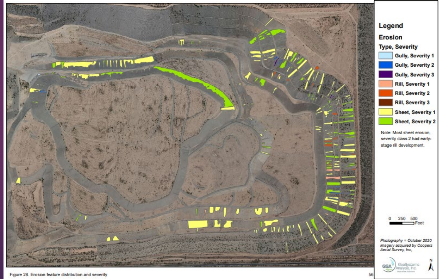
Figure 28. Erosion feature distribution and severity
