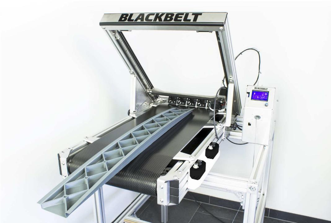
The **BLACKBELT 3D printer** is a new type of 3D printer using fused filament fabrication in combination with a unique belt technology. Printing on a belt (patent pending) provides new possibilities, like long prints, printing horizontal overhangs without support and producing series production of same or individual parts.
